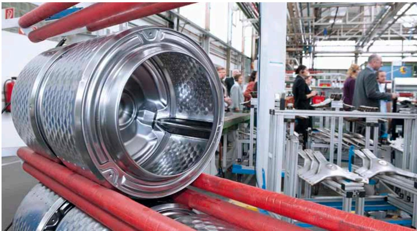
*The honeycomb drums are created in special machines manufactured especially for this purpose.*
